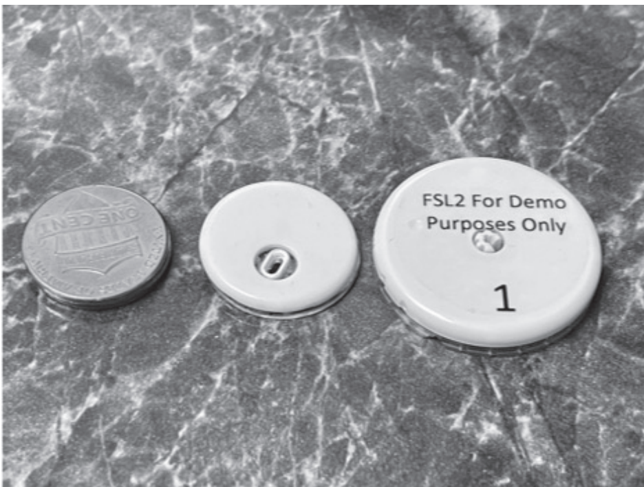
Figure 1. The larger object on the right is the transmitter for the Libre 2 glucose sensor, the middle one is the transmitter for the Libre 3.
